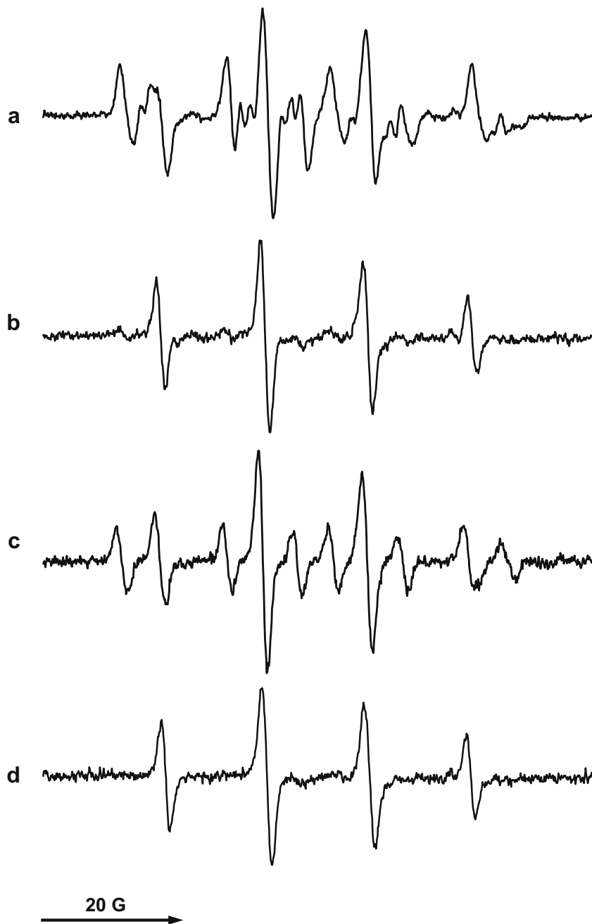
Figure 7. Comparison of iron-dependent formation of methyl radical spin adducts from the spin traps CADMPO, DMMCAPO, CAEMPO, and EMMCAPO. (a) A Fenton system was used with the following initial concentrations: CADMPO (40 mM), \text{FeSO}_4 (1 mM), EDTA (2 mM), \text{H}_2\text{O}_2 (0.2%) in 20% aqueous DMSO. The reaction was stopped after 10 s by 1:1 dilution with phosphate buffer (300 mM, pH 7.4, containing 20 mM DTPA) and the spectrum was recorded using the following spectrometer settings: sweep width, 80 G; modulation amplitude, 0.21 G; microwave power, 20 mW; time constant, 0.08 s; receiver gain, 5 \times 10^4 ; scan rate, 57 G/min. (b) Same as in (a), except that DMMCAPO was used. (c) Same as in (a), except that CAEMPO was used. (d) Same as in (a), except that EMMCAPO was used.
